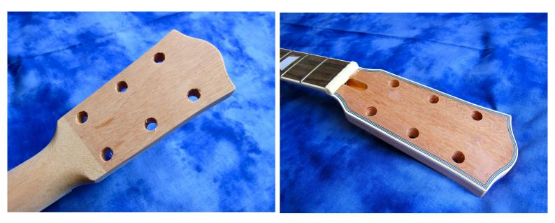
The mahogany neck features a separate headstock, glued on just beneath the bottom tuner holes. The headstock's front is spruced up by a mahogany veneer and multiple black-and-white binding.
