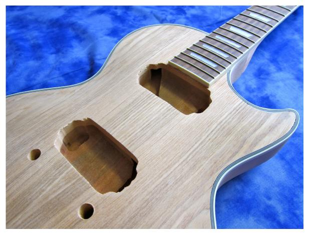
The pickup routs look a bit rough, but the untidy edges will be covered by the pickups and their bezels.
